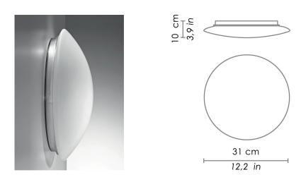
Wall-ceiling lamps with diffuser in mouth-blown, satin-finish opal triplex glass; chlorine-resistant, anti-UV, neutral translucent polycarbonate frame. Twist-lock system for the glass component. The product is suitable for indoor use only. IP44 rating.
